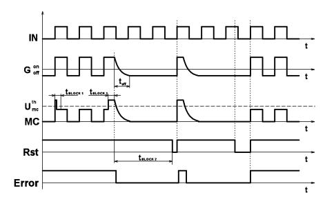
R<sub>st</sub> – Periodical internal signal of "emergency" reset
