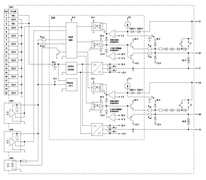
Figure 2- Functional driver circuit and turn-on circuit
