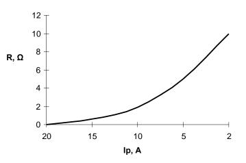
Figure 8 – Output pulse current versus gate resistor nominal
