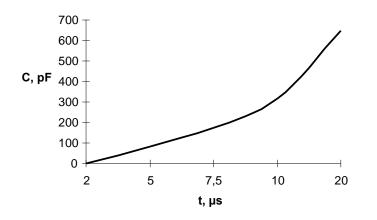
Figure 9 – Turn-on delay time of saturation voltage versus trimming capacitance  $C_b$  nominal
