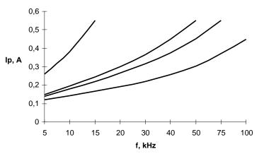
Figure 5 – Safe operation area versus frequency and gate capacitance (with gate resistor 1  $\Omega$ )
