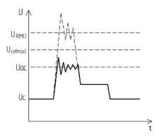
Figure 12 – Driver operation when collector-emitter overvoltage protection operate of controlled transistor where Uac – protection operate voltage against overvoltage; Uce(max) – max. collector-emitter voltage of power transistor, Ur(mc) – max. reverse voltage on collector output
