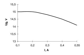
Figure 7 – Transistor gate voltage versus current consumption
