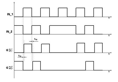
Figure 4 – Functional diagram of driver operation
