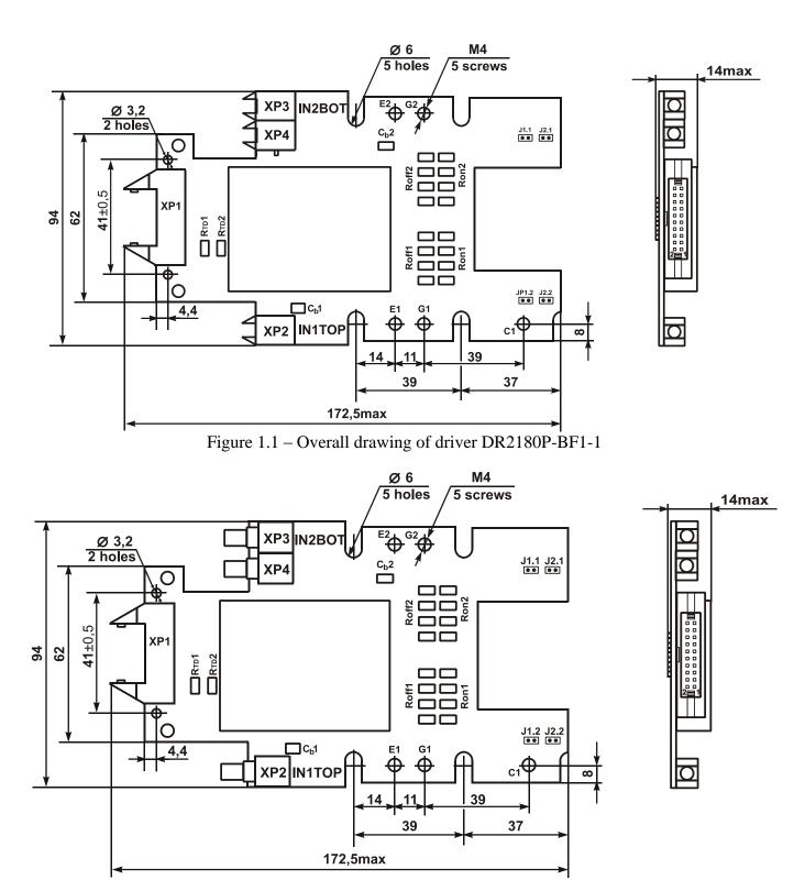
Figure 1.2 – Overall drawing of driver DR2180P-BF1-2
