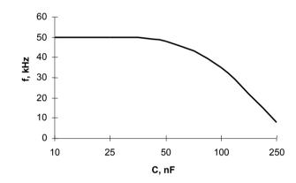
Figure 7 – Graph of rise/fall time versus gate capacity (with gate resistor 5  $\Omega$ )
