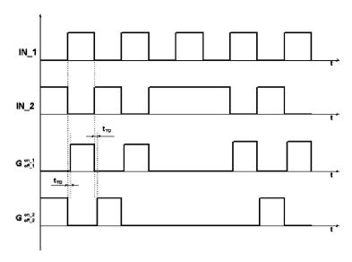
Figure 4 – Functional diagram of driver operation
