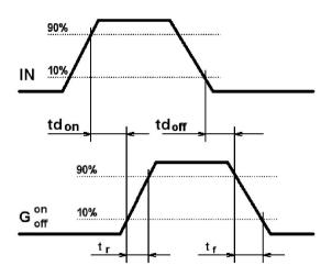
Figure 12 – Diagram explaining driver time characteristics
