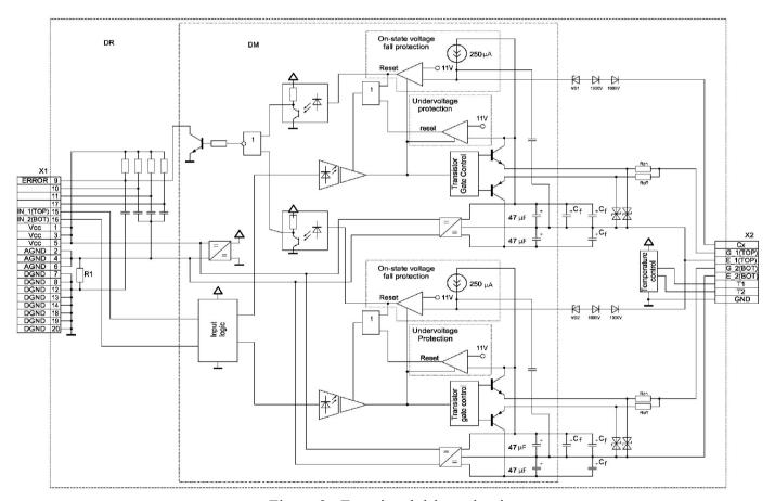
Figure 2– Functional driver circuit
