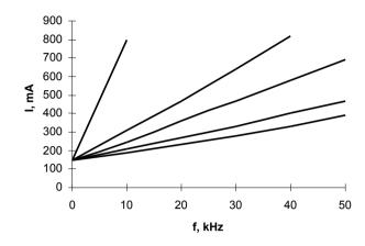
Figure 5 – Graph of driver current consumption versus no-load control signal frequency
