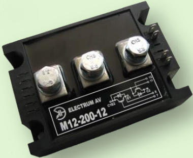
Module of rectifier bridge on Schottky diodes in diesel-generator
